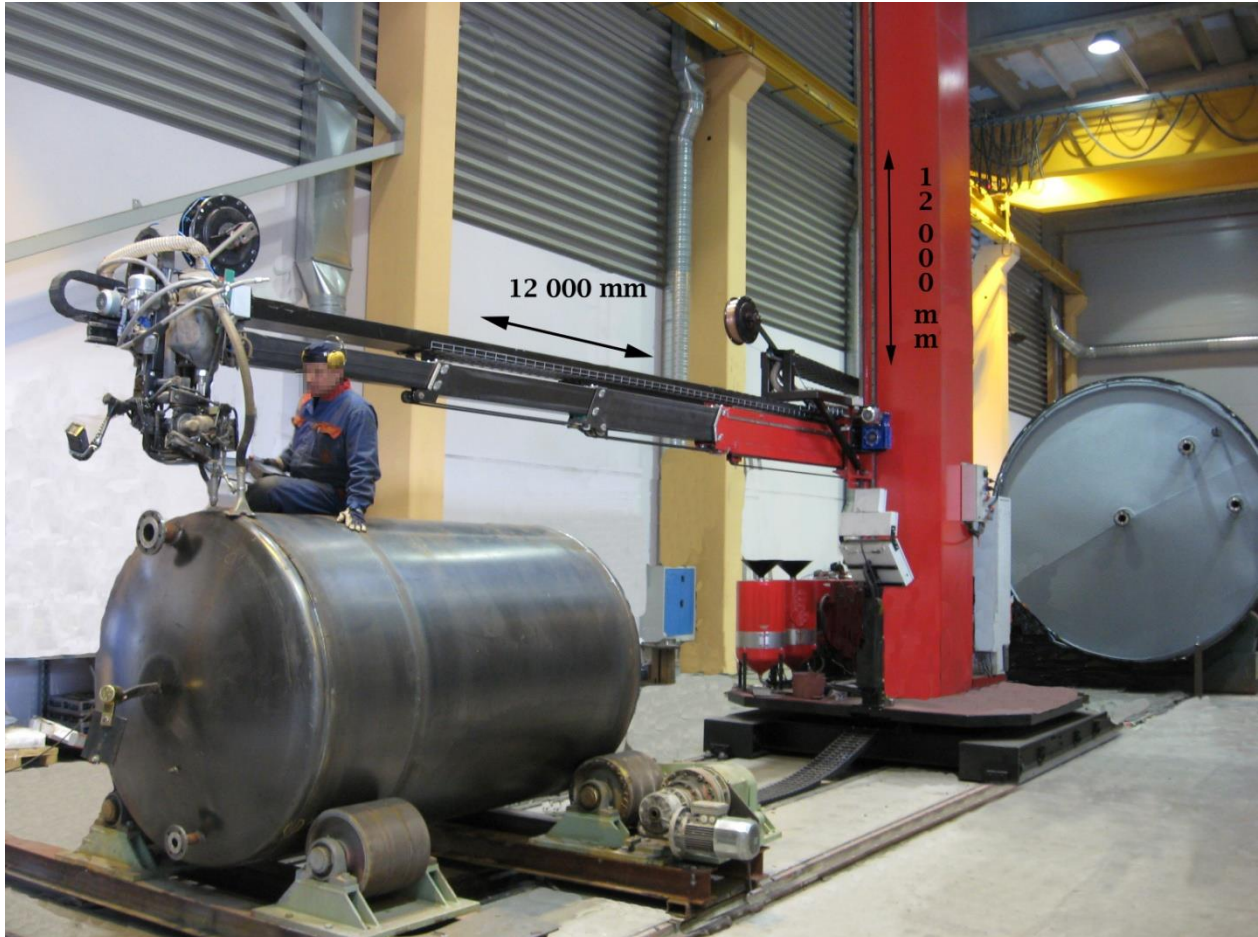
Welding Tower equipped with a telescopic beam.
