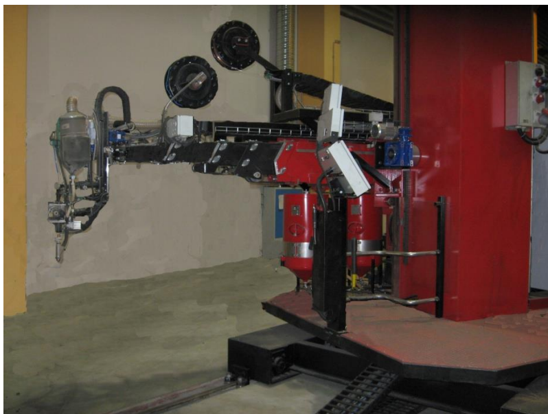
Welding Tower equipped with a telescopic beam.
